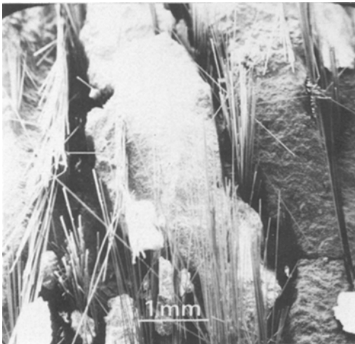
Figure 7 Delamination in grc stored for 90 days in dry air resulting from the linking of interfacial cracks with matrix shear cracks.
